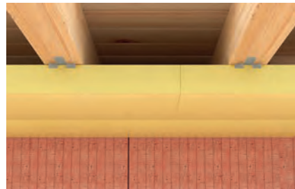
Pressure-resistant insulation boards on ceiling undersides
