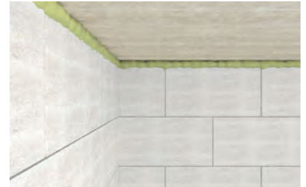
Closing joints in structural work
