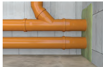
Filling pipe penetrations
