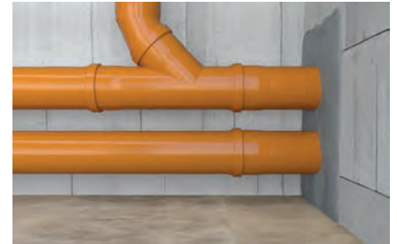
Filling pipe penetrations
