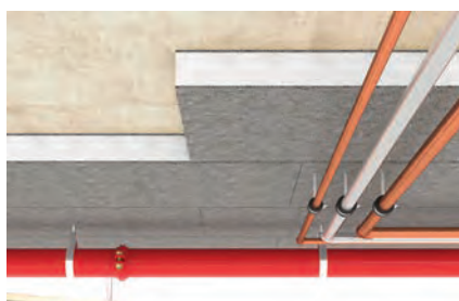
Insulation of cellar ceiling
